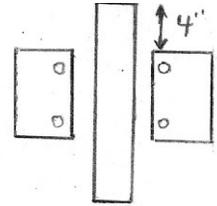
**CAUTION!! Do not over tighten 1/4" Wing nuts as you will indent the PVC Socket making it impossible to get the Dryer into Socket after assembly.**
